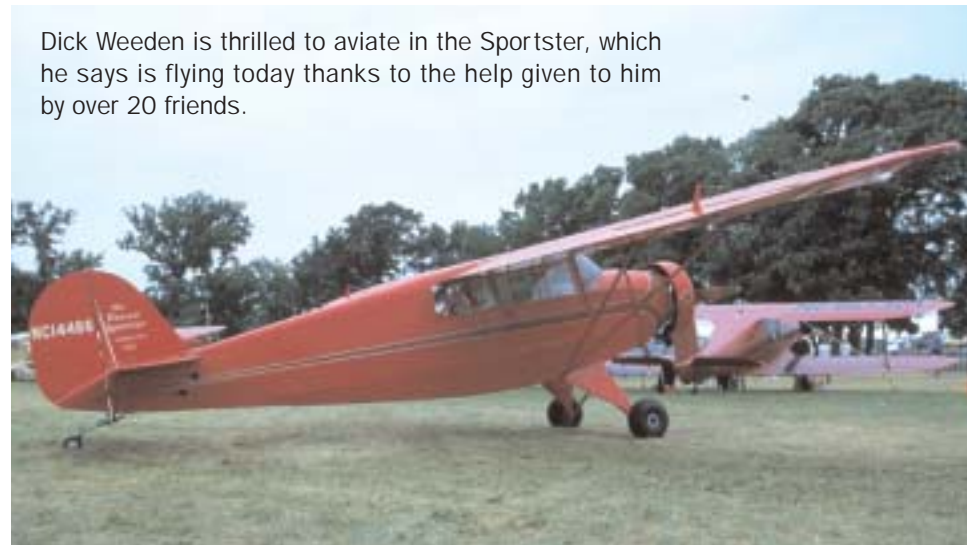
The 70 hp LeBlond motor is pretty rare, but a round engine was top of Dick’s list in desirable features for the airplane he wanted to restore.
