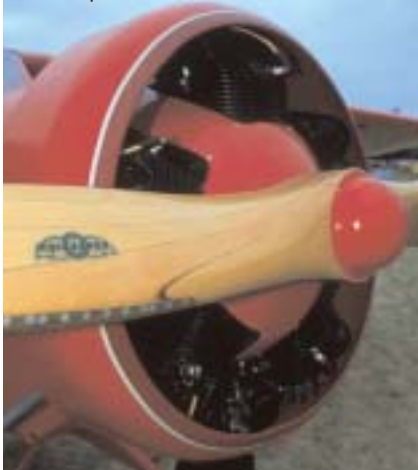
The 70 hp LeBlond motor is pretty rare, but a round engine was top of Dick’s list in desirable features for the airplane he wanted to restore.
