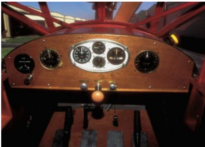
A Consolidated instrument cluster dominates the center of the instrument panel on the St. Louis Cardinal. On the far left is the Splitdorf magneto switch, with a nonsensitive altimeter to the left of the Consolidated panel, and the tachometer on the right. An original-style steel ball turn and bank is installed in the right side of the Consolidated panel.
