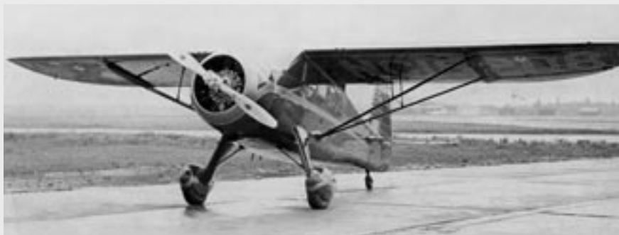
These two photos were used in the Howard Aircraft Corporation promotional publication. DGA-11 NC 18208 450 Horse Power Wasp Jr. Colors: Insignia Blue and Yukon Gold
