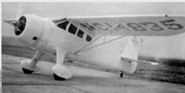
This is the "Flanigan" after it went through the factory certification. The photo was taken by me at "Muni"...The ship was later sold to Mexico along with two others. Notice the only changes from original to licensed airplane are a new fin and rudder, exhaust outlet on the left side instead of the right, rounded rear window and nav light on the fin instead of the rudder.
