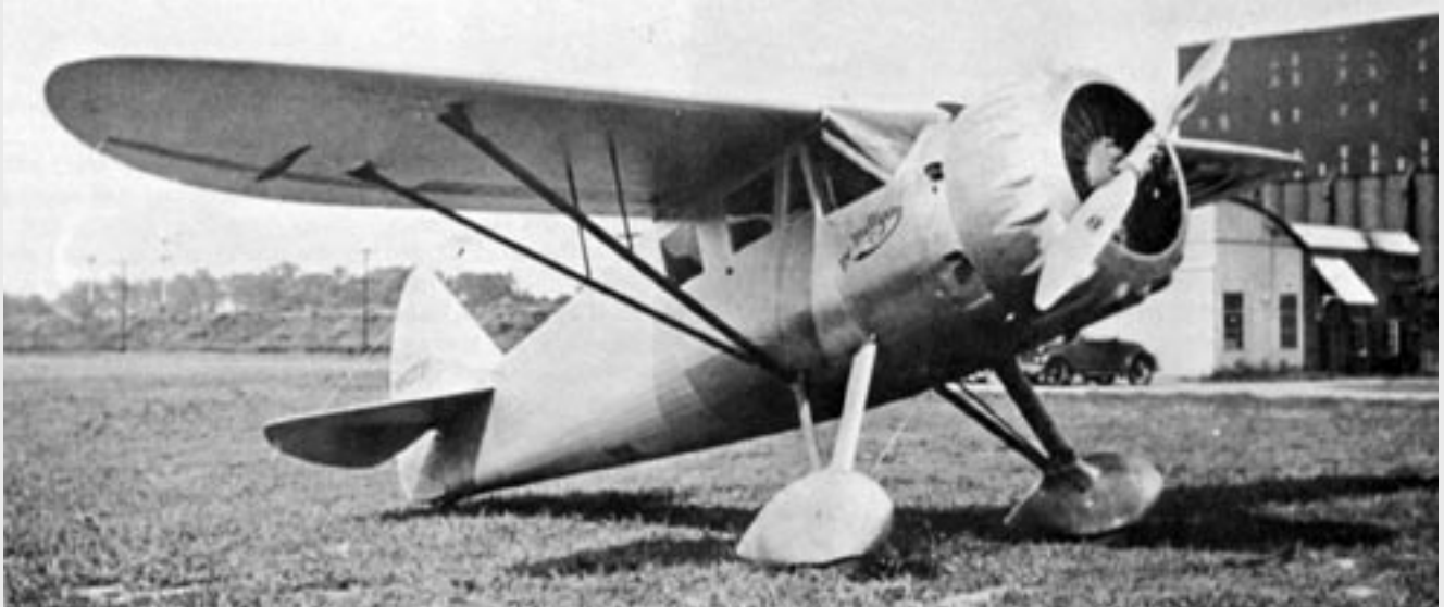
Mr. Mulligan on the day of its first flight. Few fairings had been applied at this point. The exhaust system visible in this shot is different from what appears on later photographs of the racer.
