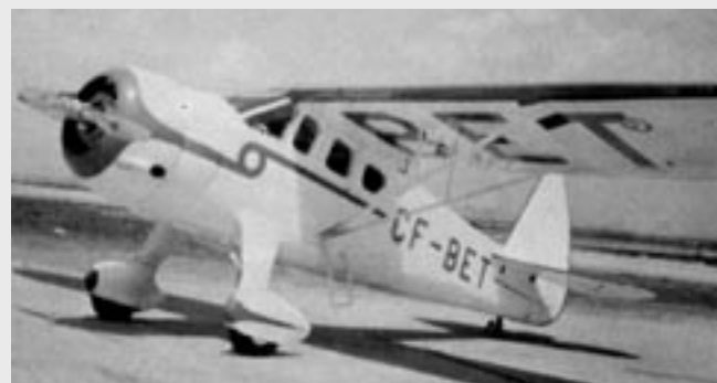
This is the first Howard seaplane. Photos taken at the factory fly-away hangar in Chicago. Note the high gear. This was a double door (left and right) model. Also, it was equipped with three fuel tanks.
