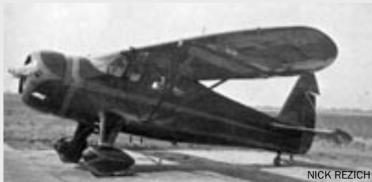
CAA DGA-8. Note the lower gear and right hand door. This airplane was loaded with radio gear for CAA work. The pilot got lost over Kansas City and cracked it up when it had only a few hours on it. Ship was rebuilt by Howard.
