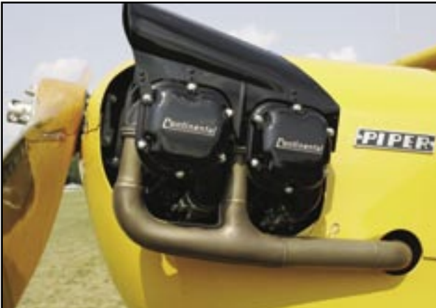
Craig's meticulous work on the Continental engine is apparent in the fit of the cowling and the "eyebrows" above each bank of cylinders.
