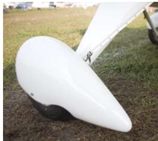
The tubular structure of the landing gear is covered with an aluminum fairing, leading to a nicely finished pair of replica fiberglass wheelpants. The small cable attached to the trailing edge of the landing gear is a safety cable. It was originally installed in case of a failure of the originally installed phenolic piston within the oleo strut. Later, after an airworthiness directive (47-20-02) and Aeronca Service Helps and Hints No. 12 required changing the phenolic part to one made of aluminum, the need for the cable was negated, but most owners keep it, just in case!
