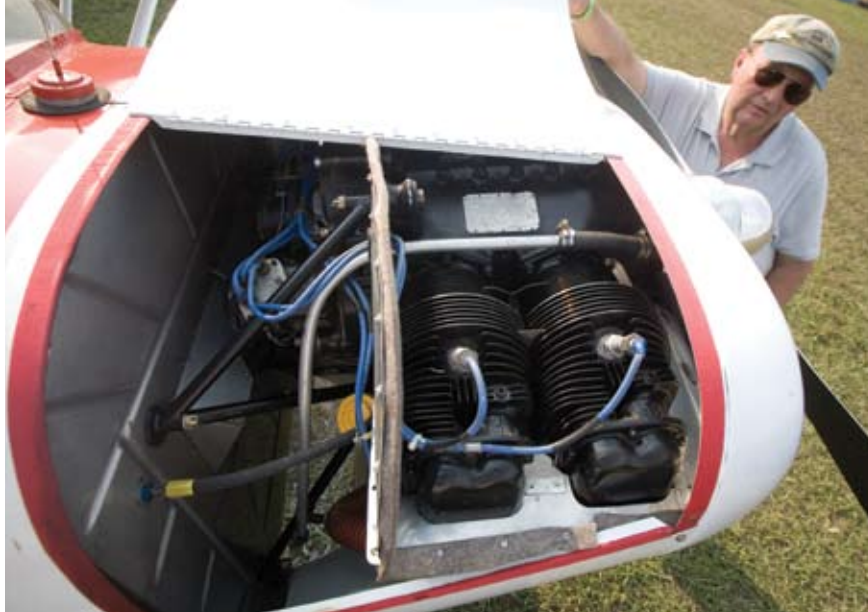
Danny Poulton holds open the top cowl to reveal the Continental C-85 installation. It appears Danny has decided not to trust his Chief mechanical fuel gauges, which are known to be troublesome, and is using an old standby, the wire and cork float gauge so common prior to World War II.
