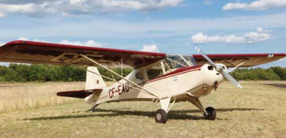
The Fleet Canuck has a distinctive narrow-waisted look to the aft fuselage. That's accentuated by the rather wide cabin that can accommodate two people in full winter dress.
