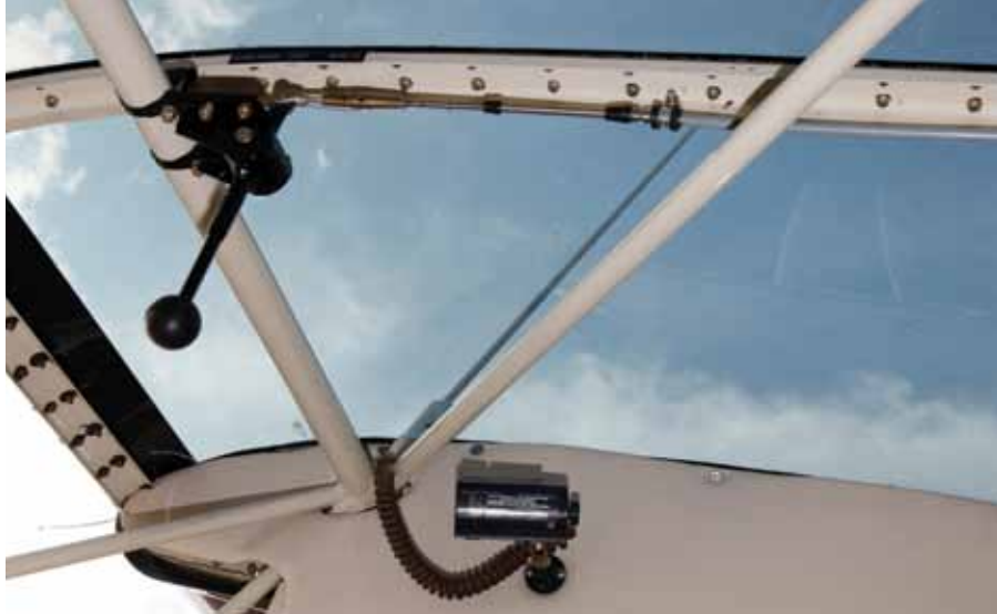
The trim system uses this handle and Teleflex cable.
