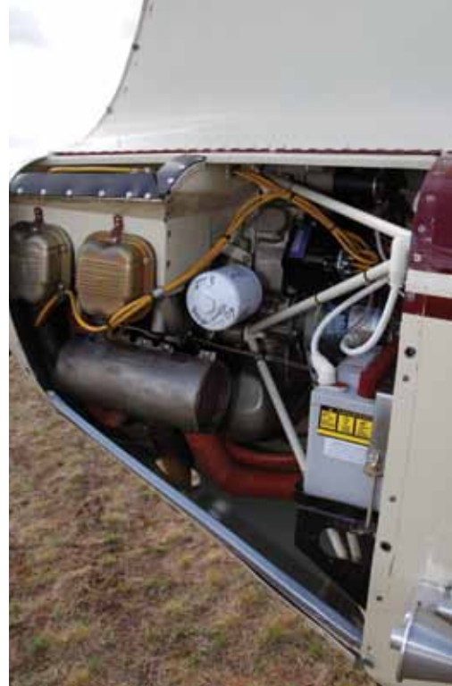
The Fleet Canuck is powered by a fuel-injected Continental C-85, and it uses bungees tucked up in the bottom of the fuselage to absorb landing loads.
