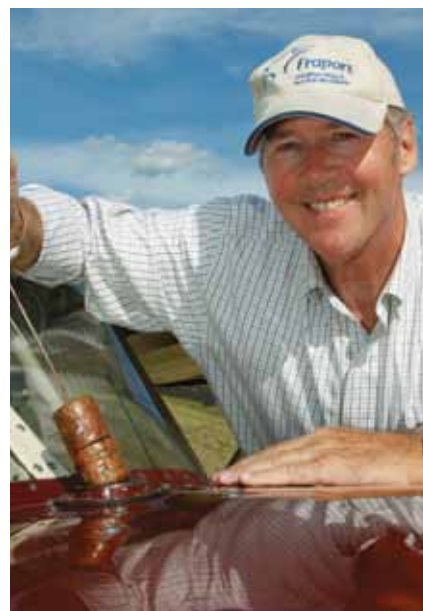
Joe Leslie and his simple fuel gauge familiar to most pilots, a wire on a cork.
