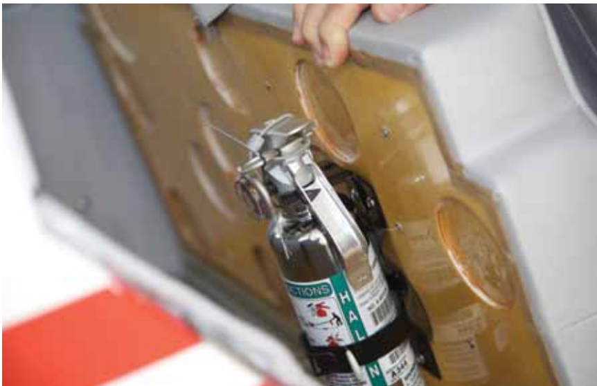
Stored under the wide rear seat of the P-12 is this chromed Halon fire extinguisher, handy during any ground emergency.
