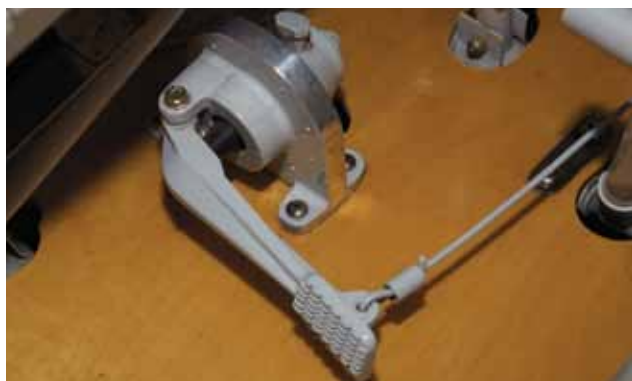
So typical of the careful restoration work done by George, the Scott master brake cylinder for the rear seat pilot has a polished mounting ring, while the rest is painted.
