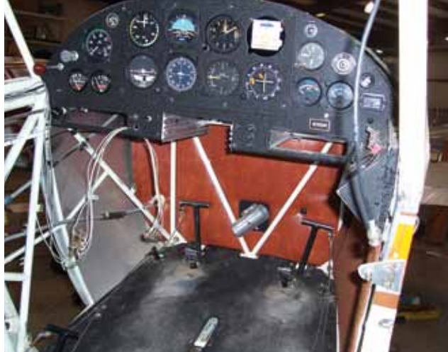
The PA-12's cockpit and instrument panel before the restoration shows the hodgepodge of holes and slots for various radios.
