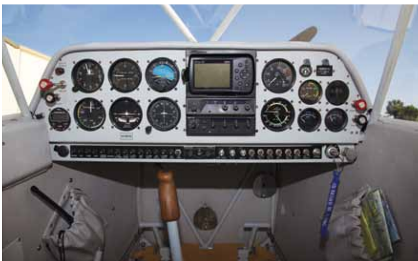
Modern avionics are compact, allowing for a tighter integration of the instrument panel. The auxiliary electrical panel on the right is gone, and the radios can now fit in a neat center stack.
