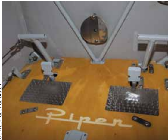
In the center of the firewall is a heat vent deflector to help diffuse the cabin air as it comes from the heat muff. A set of brushed heel plates keep the varnished birch floorboards from getting scuffed. Not using carpet makes it easier to keep the cabin clean, and keeps the weight of the furnishings down.
