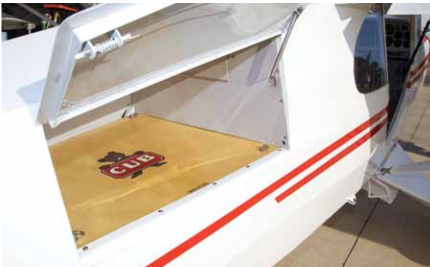
A baggage compartment on a high-wing Piper isn't complete without the Piper Cub bear, right? The coil spring door holder/opener mentioned in the text is on the upper right.
