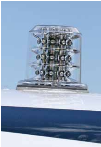
Close-up view of the new Whelen LED strobe on the fuselage, which draws less than an amp.
