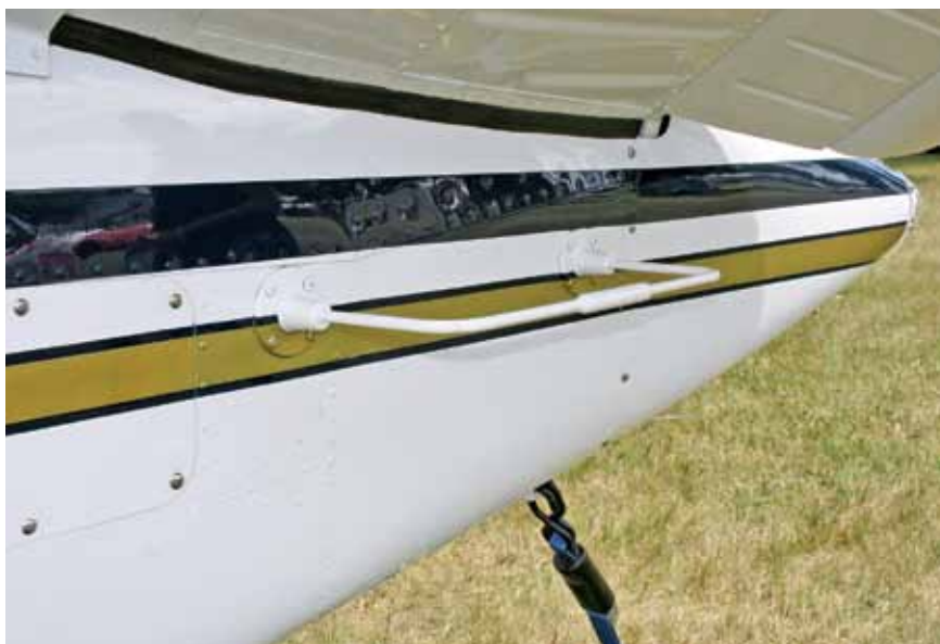
Close-up view of the old “towel bar” antenna and stinger tail mod, which is designed to give the plane a longer look.
