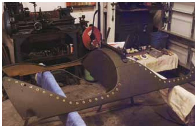
The cockpit sheet metal coaming, ready for its hand-stitched leather trim.
