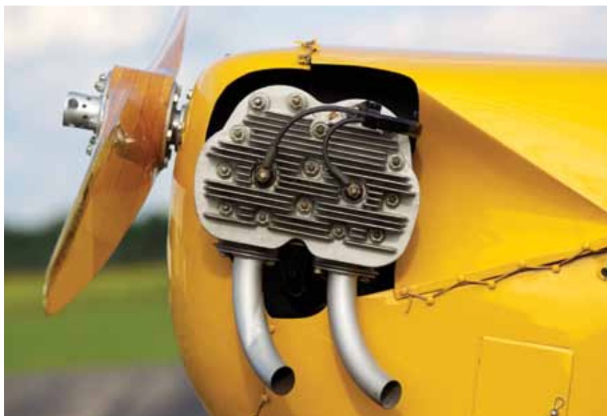
Continental’s first-production flat-opposed aircraft engine, the A-40. Unlike the later “A” series of engines, the cylinder head for each pair of cylinders is cast as one piece, as are the cylinders.
