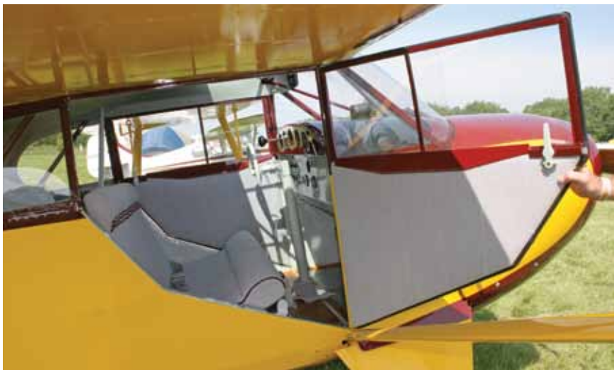
For ease of entry, the Funk brothers designed the door so it swings wide open—all the way in front of the front wing strut.
