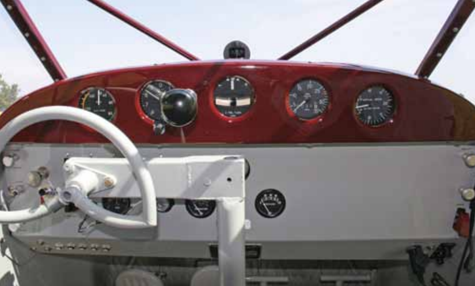
The two-tone instrument panel and the tall control column—in this instance, the right-hand portion of the yoke control has been temporarily removed to allow for passenger comfort.
