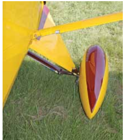
The Funk sports a pair of original wheelpants. Sometime in the 1960s the main gear was converted to Cleveland wheels and brakes.
