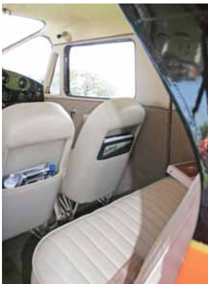
The original Switlik parachute seats were modified so they now have a roomy pocket for stowing items.
